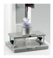
SPREAD TEST FIXTURE
